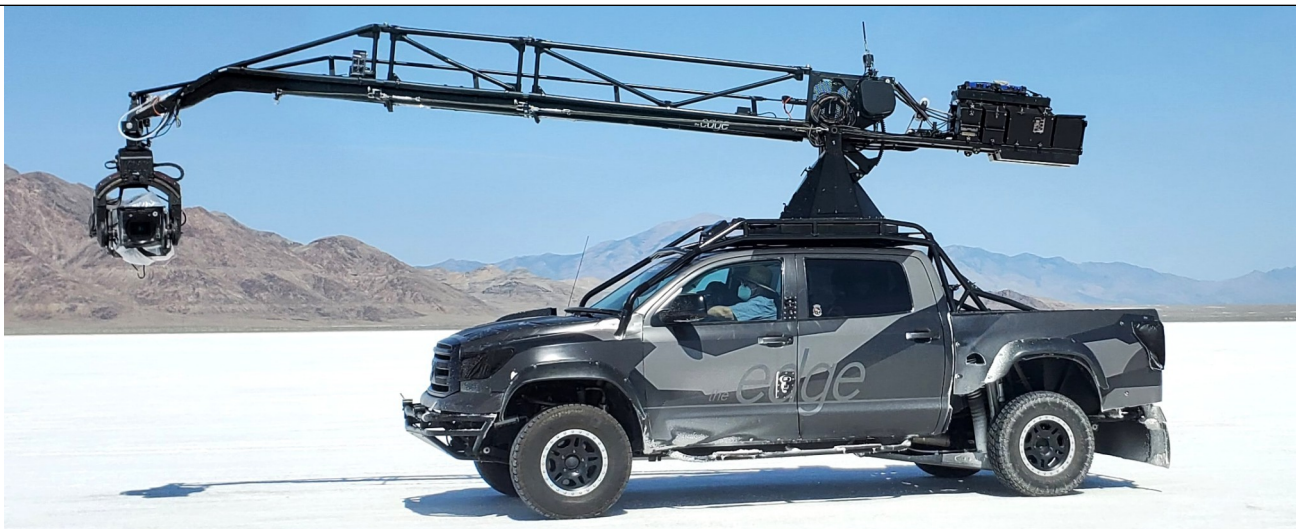
Camera Crane "Edge Crane 6" with gyrostabilized head AH-6.
