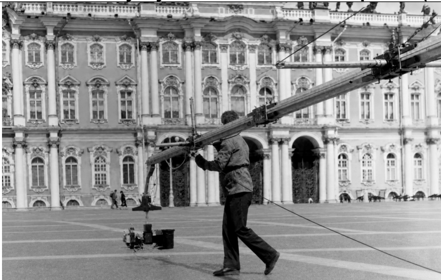
Working prototype inertially stabilized camera platform "3 GSP" developed for "chain road", cars and spring mounts.
